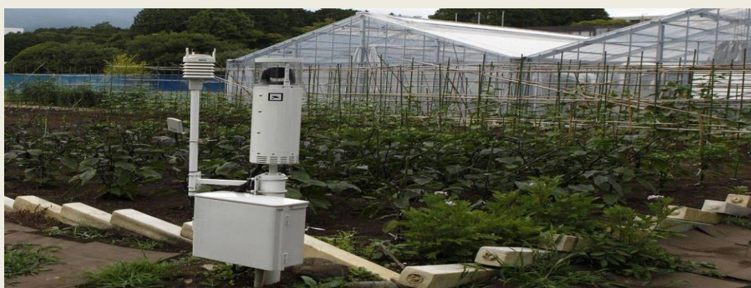
Sensors measuring temperature and humidity at a test site for Fujitsu's cloud-based farming system in Numazu, Shizuoka prefecture 58
