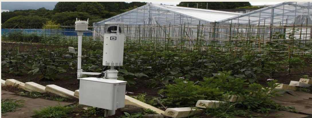
Sensors measuring temperature and humidity at a test site for Fujitsu's cloud-based farming system in Numazu, Shizuoka prefecture 5
